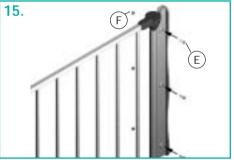
Insert 3 wall cover screws (E) through oblong holes in top, middle and bottom of assembly.
